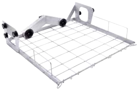
A 100 upper basket for modules • Upper basket with two docking pipes • For the connection of up to two injector modules or inserts • Automatically self-sealing docking valves • H 141, W 528, D 525 mm
