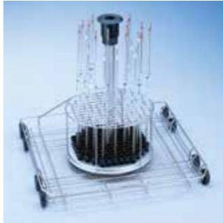
E 406 mobile injector unit • For 116 pipettes up to 450 mm • Compartment size 16 x 16 mm • Complete with retaining frame, height 150 mm • Without holder for ML/2 magnetic strip for automatic mobile unit recognition/spray arms sensing
