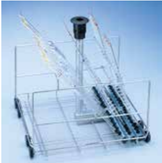
E 404/1 mobile injector unit • For 38 pipettes in 3 rows: Row 1: 10 pipettes 100 ml (length up to 550 mm), Spacing 20 mm, Row 2: 14 pipettes 25 ml, Spacing 26 mm Row 3: 14 pipettes 10 ml, Spacing 26 mm • Without holder for ML/2 magnetic strip for automatic mobile unit recognition/spray arm sensing
