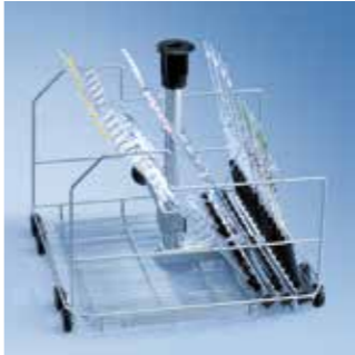
E 405/1 mobile injector unit with drying connection • As E 404/1 • Connection for hot-air drying unit • With holder for ML/2 magnetic strip for automatic mobile unit recognition/spray arm sensing
