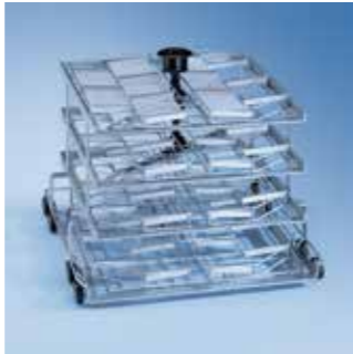
E 493 load carrier • For use in PG 8536 • For 8 x E 494 inserts for micro-titre plates on 4 levels • To ensure optimum wash results, the lower spray arm should be replaced with the enclosed flange • Clearances from bottom: Level 1: 70 mm Level 2: 85 mm Level 3: 85 mm Level 4: 90 mm
