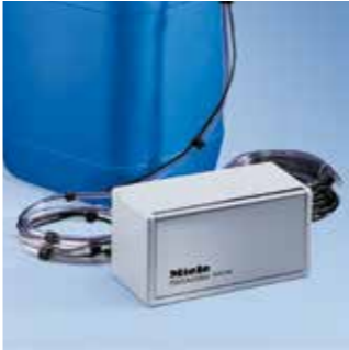
DOS G 60/1 dispenser module • For liquid alkaline detergents and chemical disinfectants • Peristaltic pump, adjustable via machine controls • Short siphon (200 mm) for 5 l canister incl. level monitoring • Length of connection lead: 1.90 m
