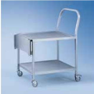
MC/1 Mielcar, supply and disposal trolley • For loading lab washers and handling baskets and inserts • 4 wheels, of which 2 are lockable • Infinitely height-adjustable • 2 shelves (trough design), handles and docking panel • Docking height: H 640–885 mm, infinitely adjustable • For G 7882, G 7882 CD, G 7892 and PG 8535 only in combination with plinths (H 30 cm) • H 1000, W 630, D 814 mm (with docking plate raised D 960 mm)
