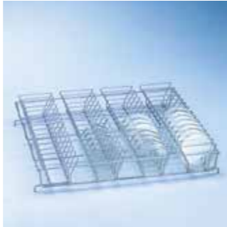
E 137 onsert 1/1 for E 136 • For 56 Petri half-dishes, 100 mm • 56 holders, Height 70 mm • Spacing approx. 26 mm • H 95, W 485, D 445 mm
