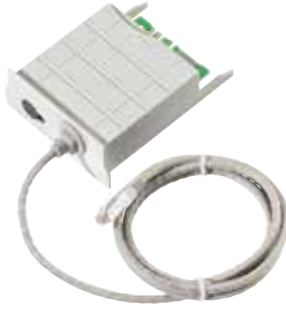
Ethernet module XKM 3000 L Med • Communication module for connection to Segosoft Miele Edition or other process documentation software • Ring buffer for up to 30 process protocols and 2 graphic protocols • No additional components needed for direct or network connection • Supports DHCP (Dynamic Host Configuration Protocol) facilitating automatic selection of network parameters • Ready for Remote Vision (automatic reporting of faults) • Baud rate: 10/100 Mbit/s • Length of supply lead: 1.5 m • Cable can be extended • Optional for models PG 858x, PG 859x and PG 858x CD.
