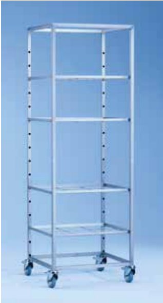
MT Mieltrans trolley • Trolley for storing and transporting baskets and inserts • 4 levels, each height-adjustable by 102.5 mm • 4 lockable wheels • Loading dimensions: 549 x 599 mm • H 1985, W 616, D 662 mm
