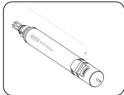
2 Install the Central Wiper on to the sonde bulkhead followed by the smart sensors.
