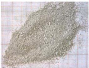
Fig. 4: Mud sediment sample after grinding in PM 100 for 5 min.
