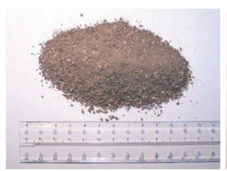
Picture 1: Pre-crushed sample
