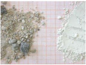
Fig. 2: Slag sample before and after grinding in PM 100 for 5 min.
