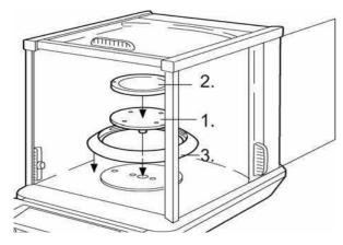
Carrier of weighing plate, attach weighing plate and circular screen in order.
