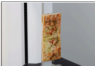
Pizza Tensile Fixture Quantifies cooked pizza firmness by measuring the tensile force and deformation distance to break sample. TA-PTF F M
