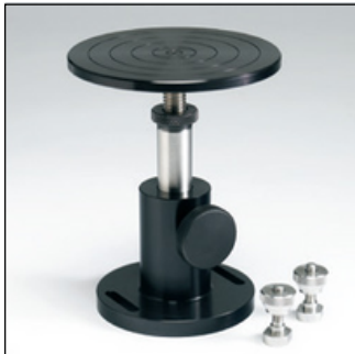
Rotary Base Table Provides quick and easy height adjustment to accommodate samples of various sizes. Included are pair of T-bolts for securing Rotary Base Table to slot in base of CTX Texture Analyzer. TA-RT-KIT
