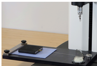
Sliding Friction Jig Measures the coefficient of friction for packaging materials according to ASTM D1894. TA-SFJ M D
