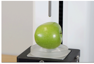
Circular Support Fixture Provides support for round samples and retains any potential fluid expressed during the test. Fixture Base Table required. TA-CSF
