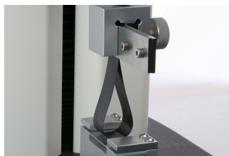
Loop Tack Test Measures the adhesive strength of pressure sensitive tape and stickers according to ASTM D6195. TA-LTT M
