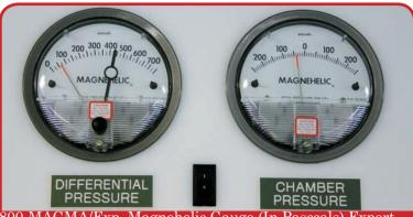
800-MAGMA/Exp, Magnehelic Gauge (In Pasccals) Export 800-MAGMA, Magnehelic Gauge (In Inches of H20) These gauges are used to monitor filter effectiveness and
