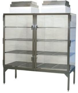
Drying cabinet with HEPA filtered flow.
