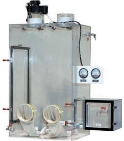
Containment glove box with double HEPA filtration package.
