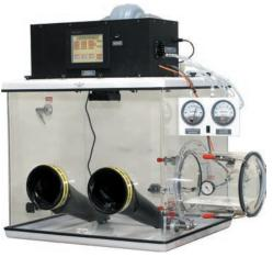
Negative pressure HEPA filtered glove box with temperature, humidity, and oxygen control. For Tuberculosis type research.
