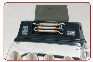
The 850-NBB Nitrogen Dry Box includes the drying train system with six (6) canisters filled with molecular sieve.
