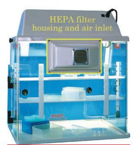
825-PCR/HEPA NOTE: HEPA housing on rear wall.
