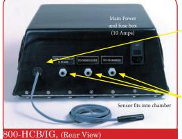
Outlet hole for Rh sensor line. Sensor fits into glove box or isolator.
