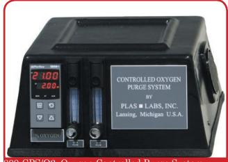
800-CPS/O2, Oxygen Controlled Purge System Front view
