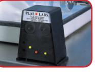
**800-AS/SPI**, Anti-Static Ionizer. Emits alternating positive and negative ions, removing static inside the glove box. This is a non-air assisted static eliminator, (no blower / no fan). The 800-AS/SPI is perfect for working with fine powders and chemicals.
