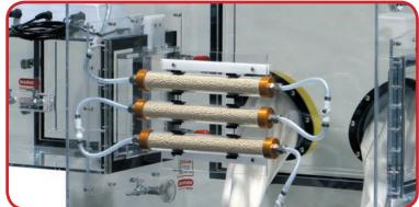
**800-DT**, Drying Train System for humidity reduction. Includes three (3) canisters filled with molecular sieve, quick disconnects, and vacuum pump.
