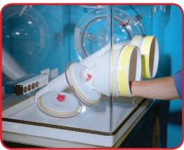
Insert plug into port opening and rotate red knob (tighten) until port is sealed.
