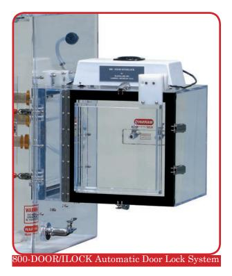
This automatic door locking system prevents both transfer chamber doors from being opened at the same time. If one door is opened, the other door is locked in five (5) seconds. The locking mechanism is rated at 120 Lbs of force. This is for operator safety. It operates on a 12 volt system. Power supply is included.
