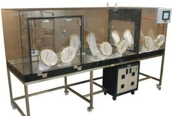
Automatic Rapid Purge Down glove box for packaging in low moisture (< 1% Rh).
