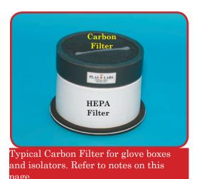
• **#800-HEPA/CARB**. Combination HEPA and Non-Impregnated Carbon absorbs most aliphatic and aromatic hydrocarbons, solvents, organic vapors, aldehydes, keytones, alcohols, organic acids, esters, sulfur compounds, and odors.
