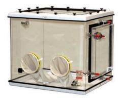
830-CP/20, with flat side access door and <u>no</u> transfer chamber and <u>no</u> vent outlet.
