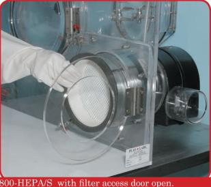
800-HEPA/S with filter access door open. Internal view (when changing filters)
