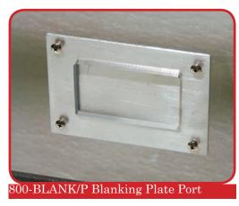
**#800-BLANK/P** BLANKING PLATE PORT. Useful for attaching special cables and plugs. This kit includes a blank aluminum plate, fastening stainless steel nuts, bolts, and sealant. The blank plate itself is ready for machining as necessary by the end user. The hole cut out is 6" x 3" (152 x 76 mm) and the blank plate is 4.5" x 7.5" (190 x 114 mm). Custom sizes are available.
