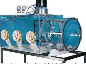
Containment glove box with 24" OD transfer chamber.
