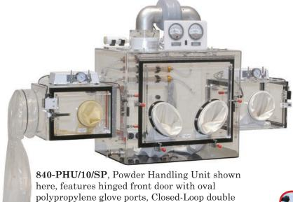
here, features hinged front door with oval polypropylene glove ports, Closed-Loop double HEPA filtration system, two clear acrylic square transfer chambers, anti-static ionizer and much more.
