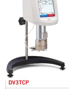
The DV3T is available in a Wells/Brookfield Cone & Plate Version Must be ordered when instrument is first purchased.
