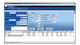
PG Flash allows users to create repeatable custom tests with all of the built-in options on the DV3T plus the addition of multiple program lines (up to 25 steps). Create the program on the PC and download to a USB Flash Drive. Upload the program from the USB Flash Drive to the DV3T.
