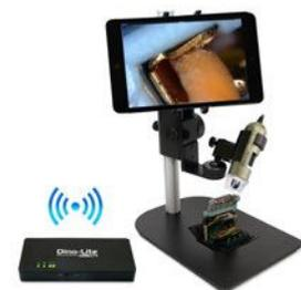
The WF-10 WiFi Streamer allows Dino-Lite USB models to be used wirelessly.
