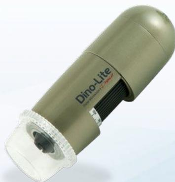
The AM4113ZT4 combines a very clear picture quality with a high magnification of 400 - 470 times. To limit glare onto the object, the AM4113ZT4 has an adjustable built-in polarization filter which fully or partially removes the reflection on glaring or (semi-)transparent materials.
