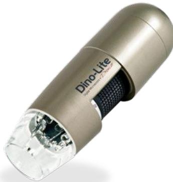
The AM4113T-FVW is suitable for inspection of paintings, ancient relics or other objects of art where UV light is required. It offers a high magnification (up to 200 times) and switchable LED lights – they can be switched from UV to white light. The UV light supplies an excitation of ~400 nm. It has a filter which blocks the returning UV light, resulting in images with natural colors.
