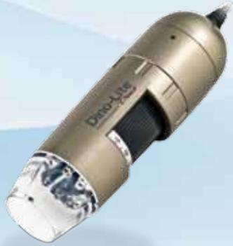
AM4113TL is one of the long working distance models and is designed to provide magnification at a greater working distance. This makes it an ideal solution for tasks where you need more working distance from the object, for example watch and jewelry repair or diamond cutting
