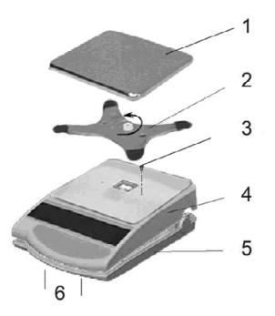
• Release both retaining hooks (6) on the lower housing section (5) and carefully remove the upper housing section (4) to the rear (please observe the upper housing section guides on the back of the balance).
