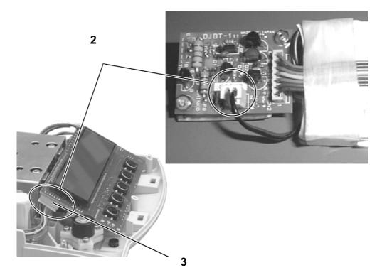
• The rechargeable battery is placed on the left side of the housing in such a way that it can be screwed onto the balance through the existing mounting using the screw (4) loosened previously. Press lightly into the housing prior to this, (there is only one correct installation possibility). Now also re-attach the display using the loosened screw (5).
