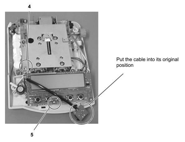
• Place the upper housing section on the rear guides and tilt forward until both retaining hooks on the lower housing section audibly lock into place. Screw down both screws to the left and right of the bracket guide tightly and resecure the bracket. Attach the weighing plate.
