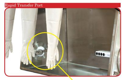
The RTP, "Rapid Transfer Port" provides containment during material transfer. For use with stainless steel transfer canister.
