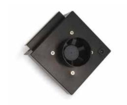
The AirShield is a separate accessory that can be purchased for any Microlab 600 instrument. It creates a positive pressure blanket of fresh air inside the pump that pushes air out over critical components on the outside of the pump, protecting them from the environment.
