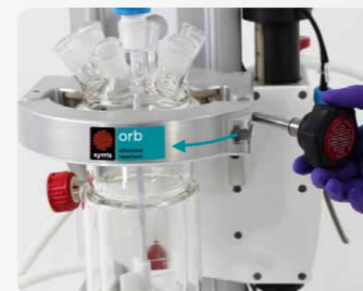
Clever clamp mechanism for quick vessel changes
