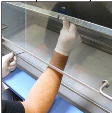
Figure 24 Lifting up the worktop against the back partition
