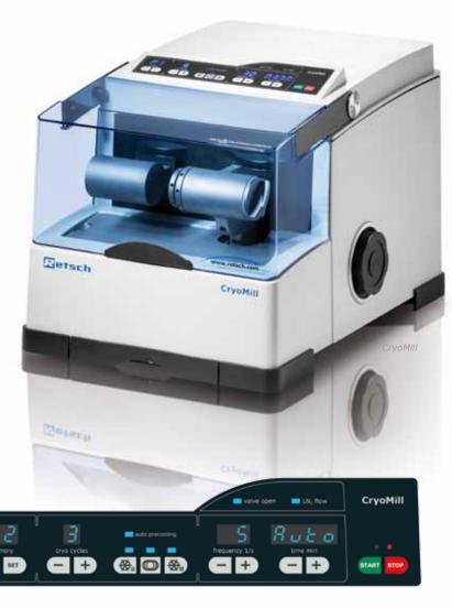
The liquid nitrogen flows through the system and is continually supplied from an **autofill system** in the exact amount which is required to keep the temperature at -196 °C. Thus the user never comes into direct contact with LN<sub>2</sub> which ensures a high degree of operational safety. The automatic cooling system guarantees that the grinding process is not started before the sample is thoroughly cooled. This results in reduced consumption and guarantees reproducible grinding results.
