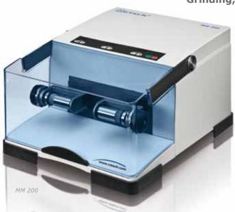
RETSCH Mixer Mills MM 200 and MM 400 are laboratory "all-rounders". They have been developed specially for grinding, homogenizing and mixing of small sample amounts quickly and efficiently. They are also perfectly suitable for the disruption of biological cells as well as for DNA/RNA extraction. The MM 400 can also be used for wet and cryogenic grinding.
