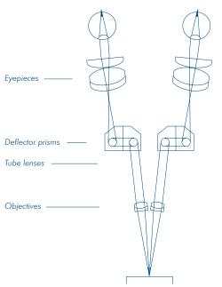
Beam path in the stereo microscope
