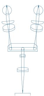
Beam path in the binocular microscope
