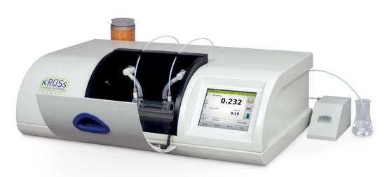
Semi-automatic sample supply with P8000-TF and peristaltic pump DS7070
