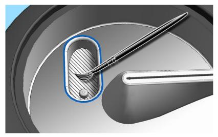
Fig. 21: Cleaning the air outlet channel
