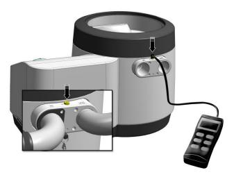
Abb. 22: Connecting the Manometer
