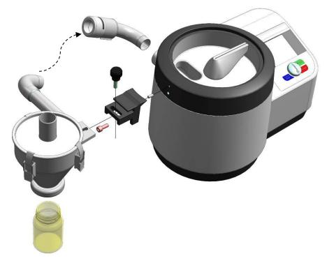
Fig. 15: Connection of the cyclone
