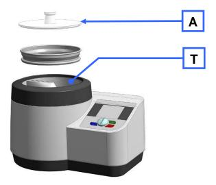
Fig. 7: Inserting the test sieve
