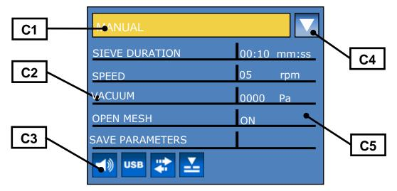
Fig. 1: View of the menu in the display unit
