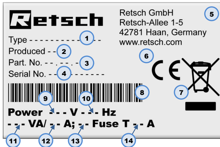
Fig. 1: Type plate lettering
